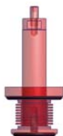
spindles – metallic bellow design
